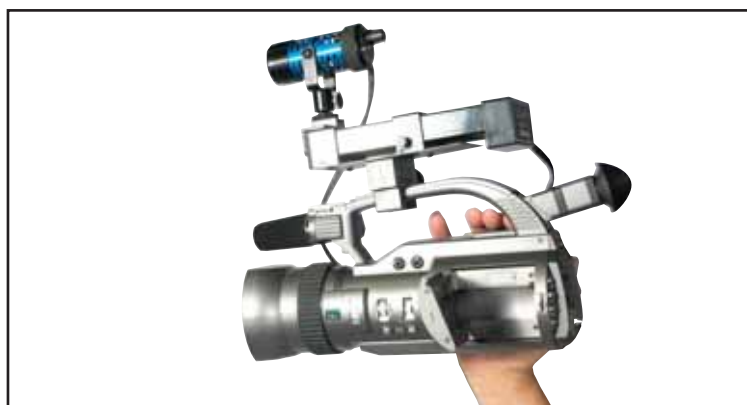
Battery on top of camera mount
